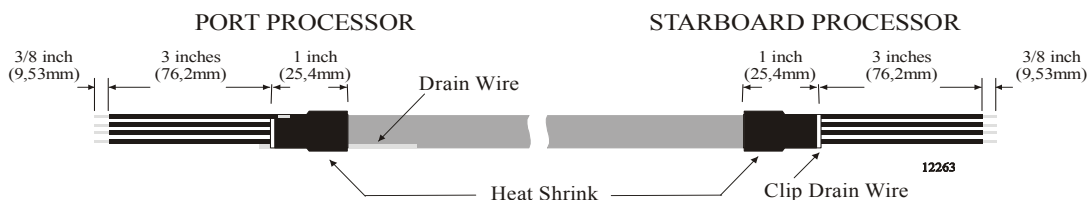
Figure 4-13: Four-Conductor Serial Communication Cable
