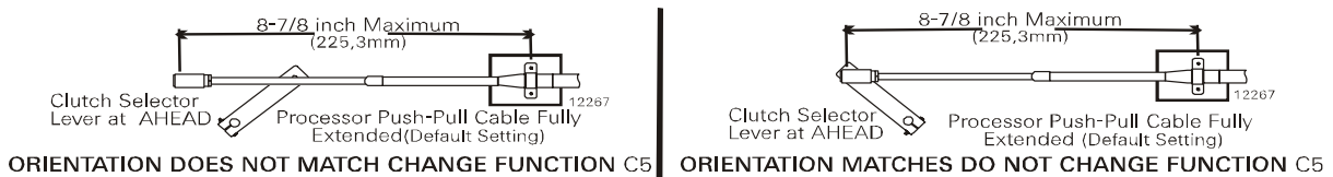
Figure 48: Clutch Push-Pull Cable Orientation
